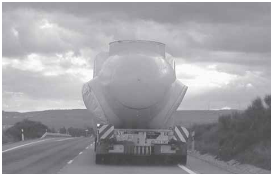
Figure 11 Transport of wind turbine nacelle.
