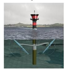
Strangford Lough. The tidal turbine is rated at 1.2 megawatts, which is enough to power a thousand local homes. It was built by Marine Current Turbines, and it will be the first commercial tidal turbine to produce energy, when it begins operation later this year.
