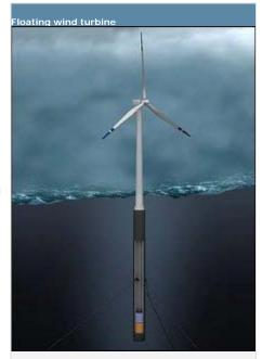
The flotation element stretches 100 metres below the sea surface
